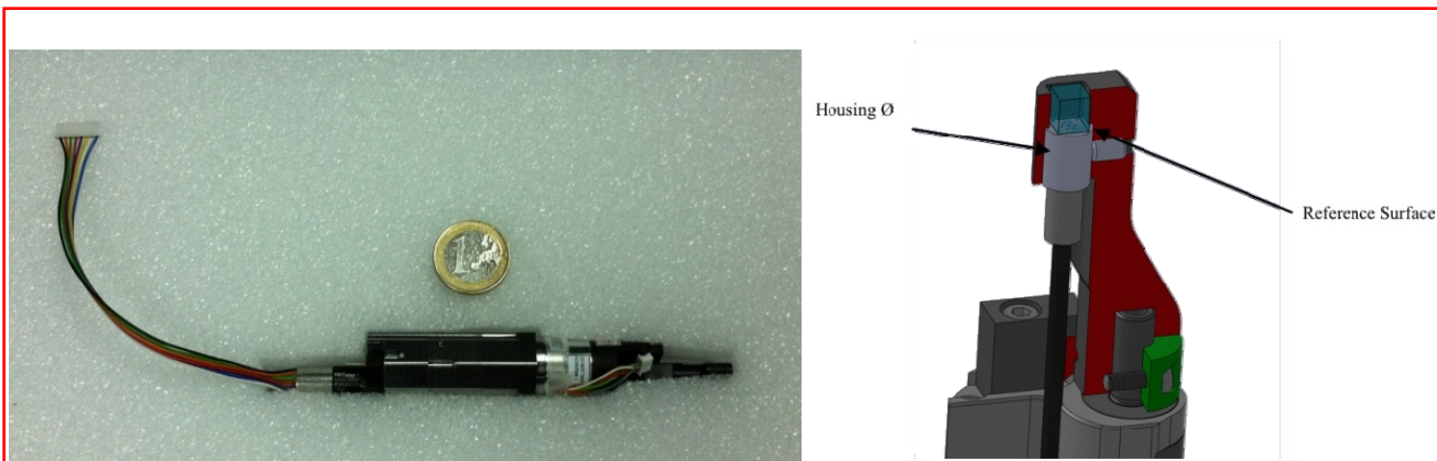
Figure 4. Left: Fiber MOS positioner prototype (December 2011). Right: Positioner button detailed design.
