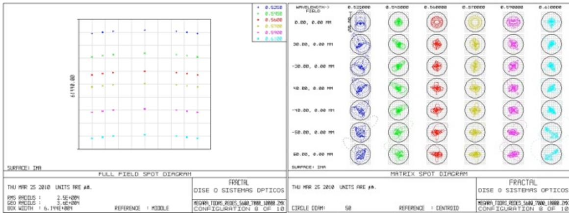
Figure 8. Left: projection on the detector of the spectra from fibers at different positions of the pseudo-slit in the configuration of the grating VPH570-5600. Right: spot diagram of the spectra from fibers at different positions of the pseudo-slit in the configuration of the same grating. Different colors correspond to different wavelengths.
