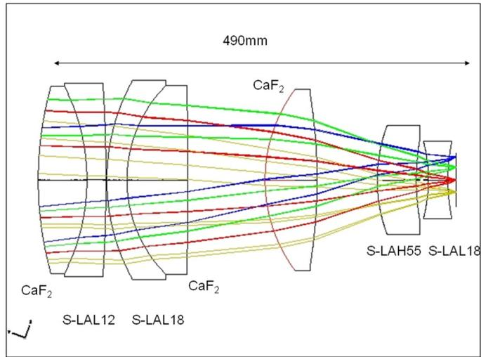
Figure 3. Camera layout. It is composed by two doublets, each of them with one CaF<sub>2</sub> lens, and three singlets.
