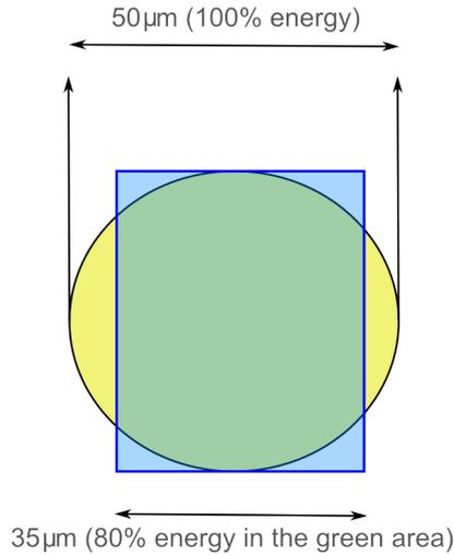
Figure 7. The value of the diameter of a circle that contains the 80% of the energy from a 100µm fiber , whose circular projection on the detector is a circle of a diameter of 50µm, is 35 µm.
