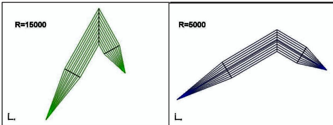
Figure 1. Example to illustrate the different angle on the grating needed for two extreme spectral resolutions with values of the resolving power, R of 15000 (left) and 5000 (right), respectively.
