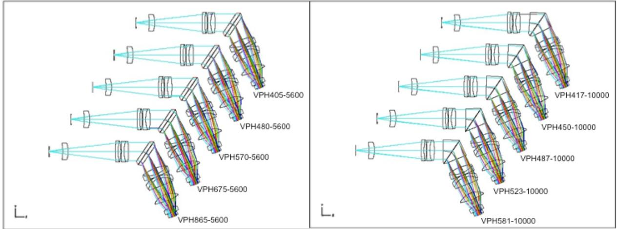
Figure 5. Left: MEGARA configuration in the low resolution mode (R=5600) where the pupil element is a VPH grating sandwiched between two windows. Right: MEGARA configuration in the mid resolution mode (R=10000) where the pupil element is a VPH grating sandwiched between two prisms to compensate the beam angle.
