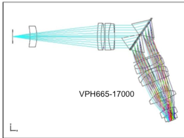
Figure 6. Design of the R=17000 grating centered at 6500 A with a pupil segmented in 2 slices [1].
