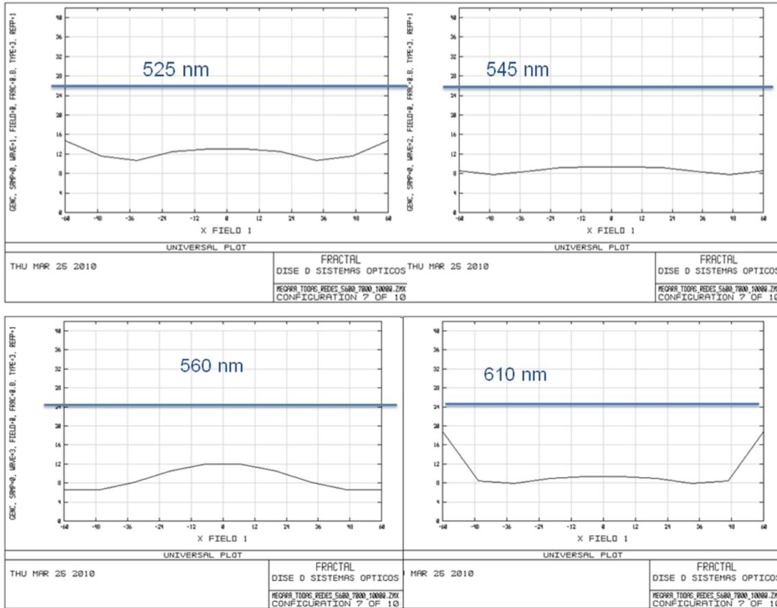
Figure 9. Four examples of the  $EER_{80}$  plots as a function of the position of the FOV (on the pseudo-slit) with the grating VPH570-5600, for the wavelengths indicated. The horizontal line represents the image quality requirement. For each configuration we obtained this kind of plots for six wavelengths, all the fields and wavelengths are within requirements.
