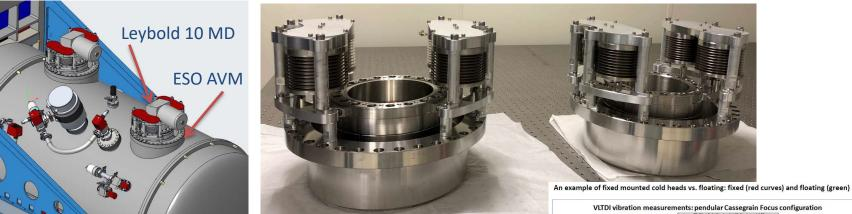
Agreement to license AVM for Closed Cycle Cooler Cold Head to **FRACTAL S.L.N.E.** AVM allows to reduce the cold head vibrations to the stability levels demanded for the instruments and the high stability demanded by the VLTI configuration. This system keeps the cold head fully floating between two soft bellows removing vibration coming from the motion of the heavy displacer.
