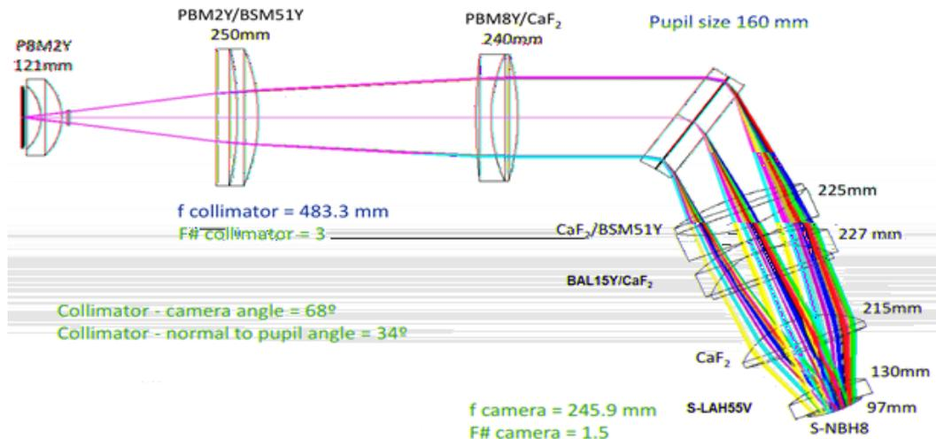
Figure 1. MEGARA optic system layout.
