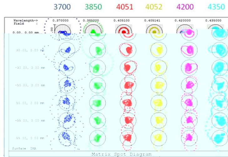
Figure 2. Spot diagram of the spectra from fibers at different positions of the pseudo-slit in the configuration of the grating VPH405-LR (LR-U). Different colors correspond to different wavelengths.
