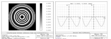
All the interferograms for final tests at the level of the collimator and camera have been simulated. The figure shows a nominal interferogram for central field (0° AOI), tilt/piston removed. The lower figure is the OPD plot.
