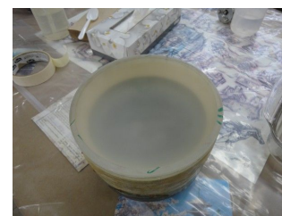
Dummy of COLL-S1 (aspheric) Diameter: 155mm
