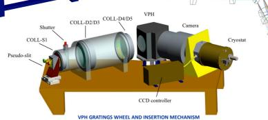
The spectrograph includes the capability of the automatic interchange of 11 VPH gratings that are placed on a Ø1880 mm aluminum alloy wheel. The mechanical mount of each VPH is screwed to a platform that has a pair of guideways screwed on its downside. These guideways are inserted on their corresponding carriages that are screwed to the wheel. VPH mounts are to be seated in a flat-cone-groove kinematic system with fine alignment capabilities on the platform.
