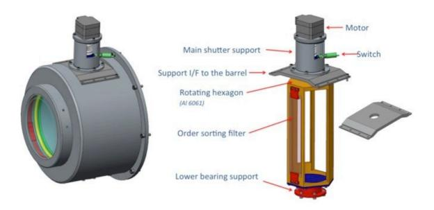
Figure 46: MEGARA shutter mechanical advanced design. The different parts of the shutter assembly are shown at right.
